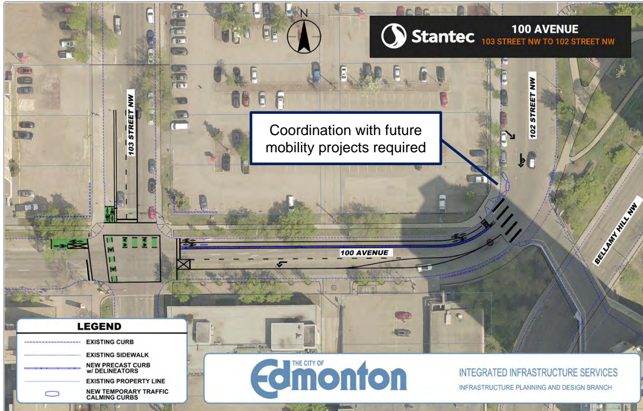
Two-way protected bike lane on the north side
